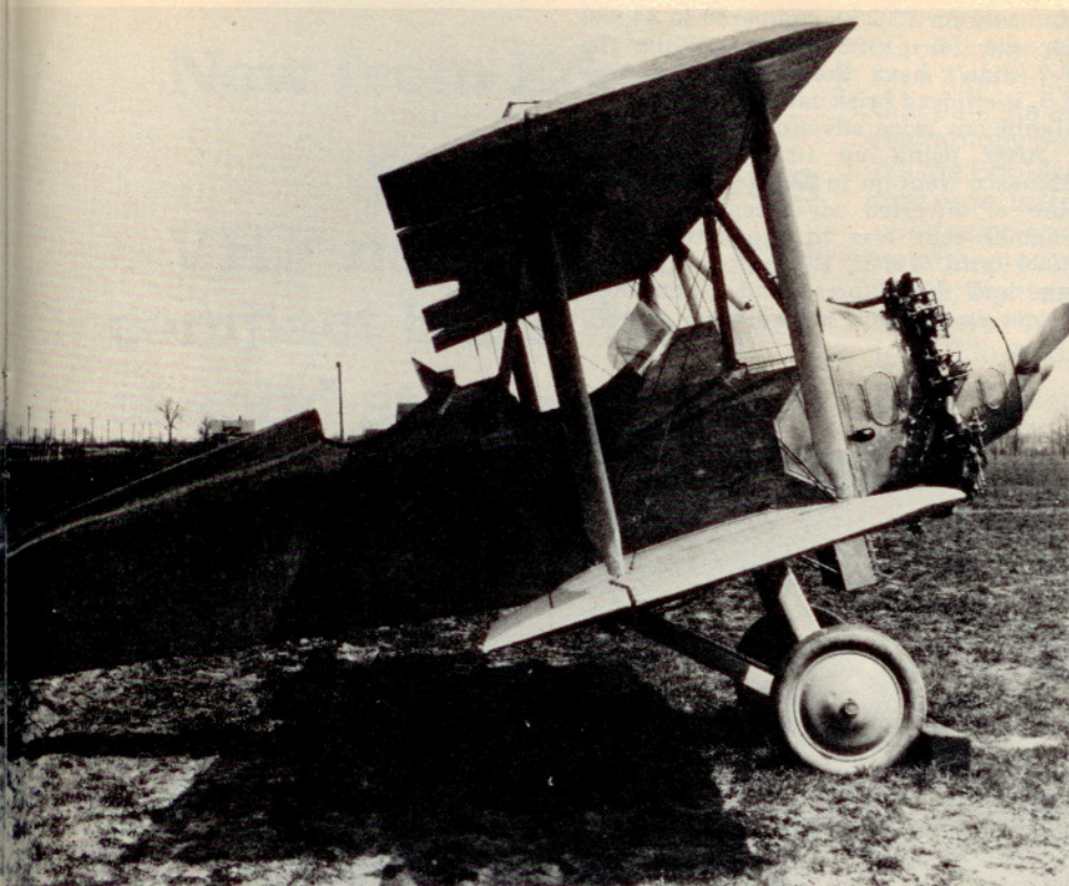
A Woodson Express with unpainted plywood fuselage in 1925. Note absence of registration numbers in that pre-regulation period and Salmson engine radiator under nose, in line with forward wing strut.
