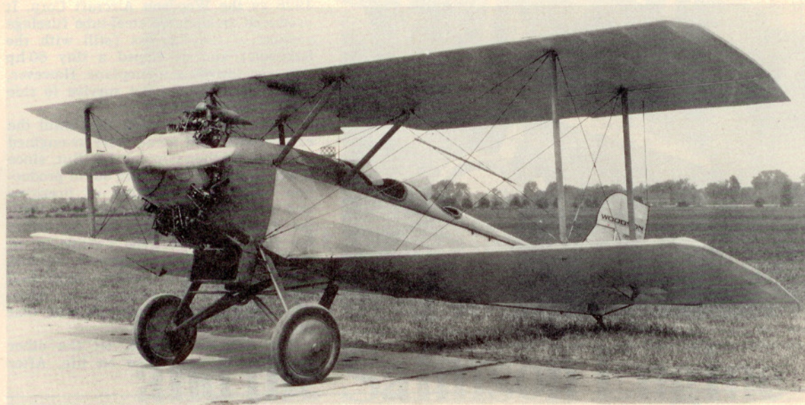
Final 1926 Express did not see production. Steel-tube design with split-axle landing gear still retained vintage Salmson engine. Notice the water header tank just behind the top cylinder. Hudek Aeronautical Collection
