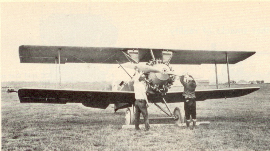
Twin radiators mounted under upper wing of Express seriously hampered visibility. Propeller is pulled from left side of airplane to start "left-hand" engine like the Salmson. Kohler photo courtesy R. H. Demmerhirt
